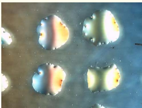
*Liquid samples (10 mL dots), imaged using the differential interference contrast (DIC) technique on our Zeiss materials microscope.*
