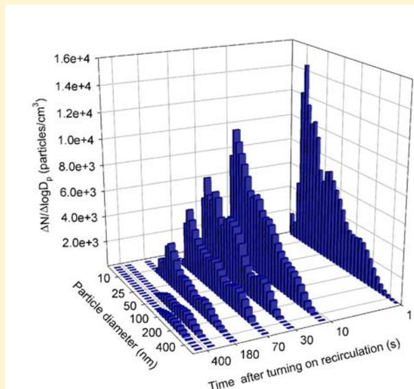
are observed for workplace air recirculation. This may be a low cost solution to reduce workers' exposure to nanoparticles in workplaces.
