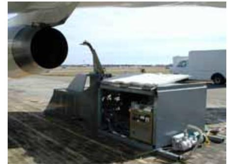
*Sampling platform for jet engine exhaust aerosol characterization experiment*
