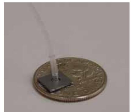
Cross section (top) and full assembly (bottom) of an adhesive-free interconnect for integrated microfluidic systems.
