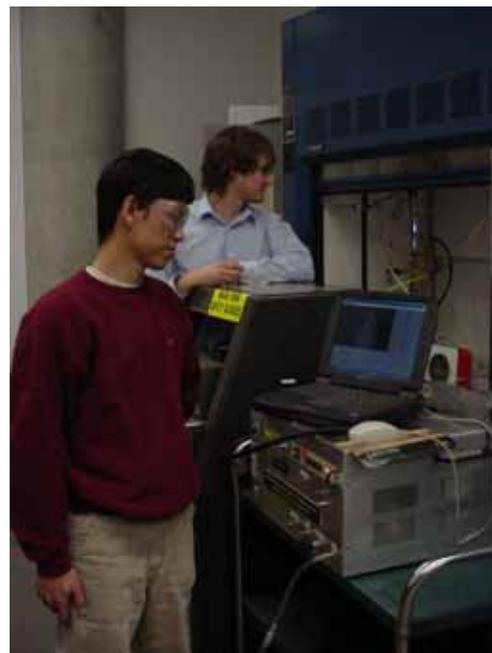
He-Shu Han and Elijah Thimsen measure the particle size distribution of silicon particles synthesized in a nonthermal plasma with the nASA
